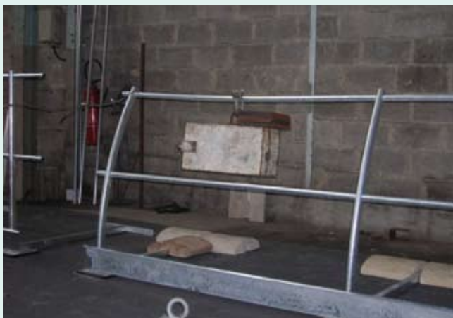
sterketest nav behalen Aboma+Keboma certificaat (neerwaartse belasting 1,25 kN).
